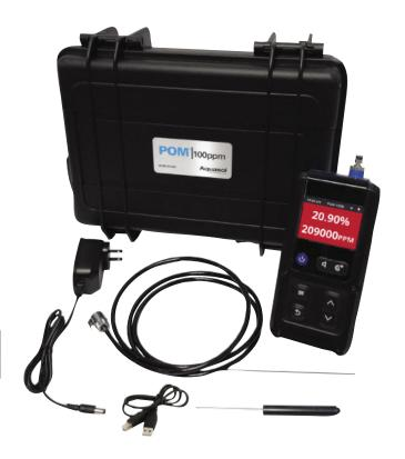
Aquasol has developed the first APP enabled handheld oxygen monitor for the welding industry. Compatible with Android, iOS and Windows. The APP allows users to monitor oxygen levels within a range of 30 metres from the actual oxygen monitor with Bluetooth transmitting capabilities.
