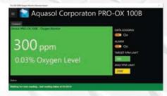
When the oxygen content reaches the operator set TARGET PPM level, the numerical value will display on a GREEN screen, a visual signal that welding can commence per the operators instructions.
