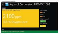
A YELLOW screen is maintained when the oxygen level falls between the maximum and target.
