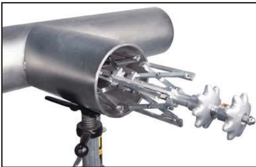
1. Tighten jaws to clamp pipe I.D.
